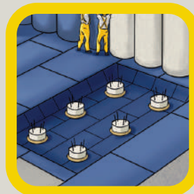
5. Underslab applications including pile caps and penetrations.
